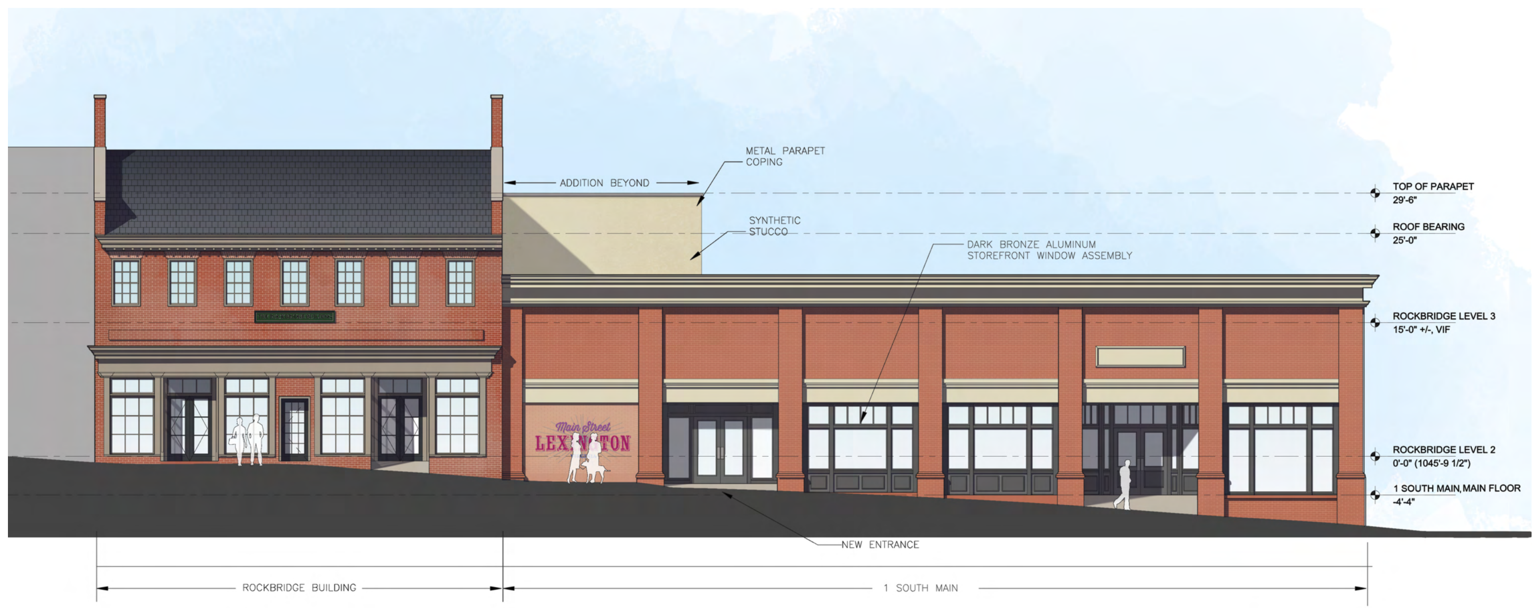
A1 EXTERIOR ELEVATION - SOUTHEAST SCALE: 3/32" = 1'-0"
