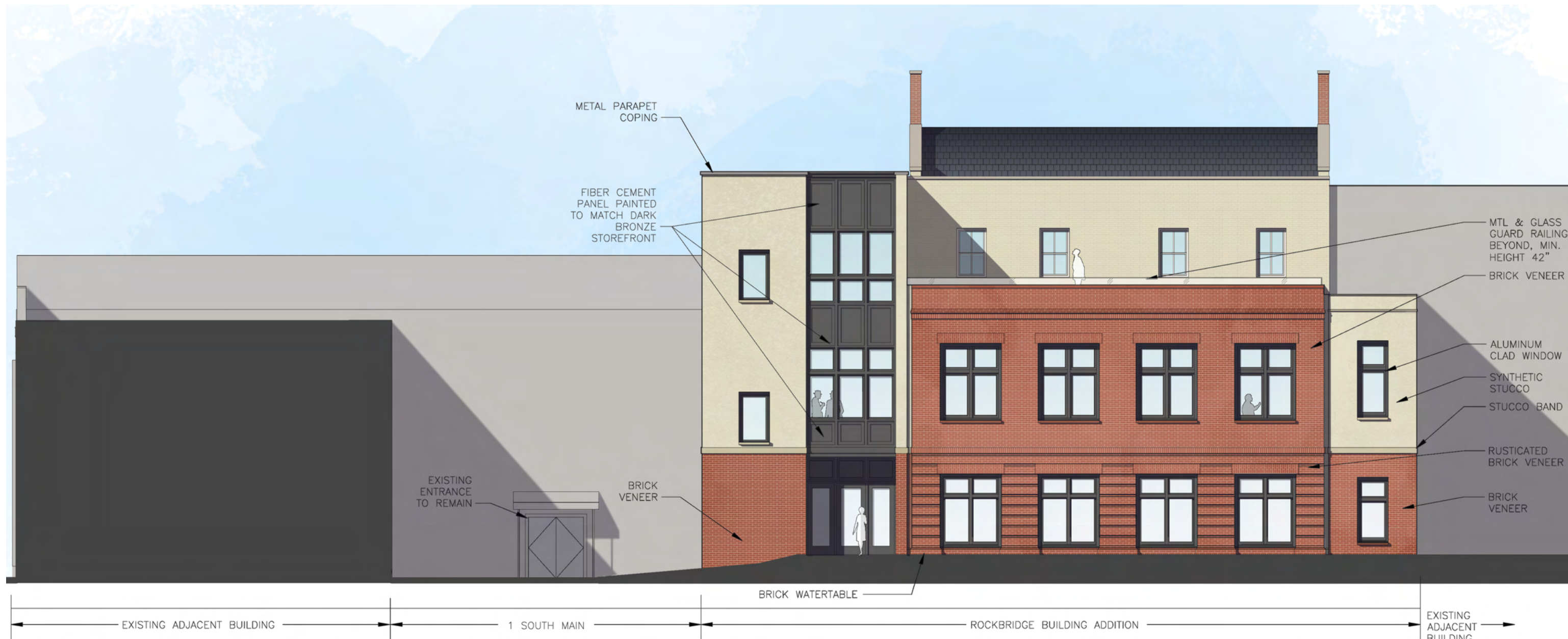
A1 EXTERIOR ELEVATION - NORTHWEST SCALE: 3/32" = 1'-0"
