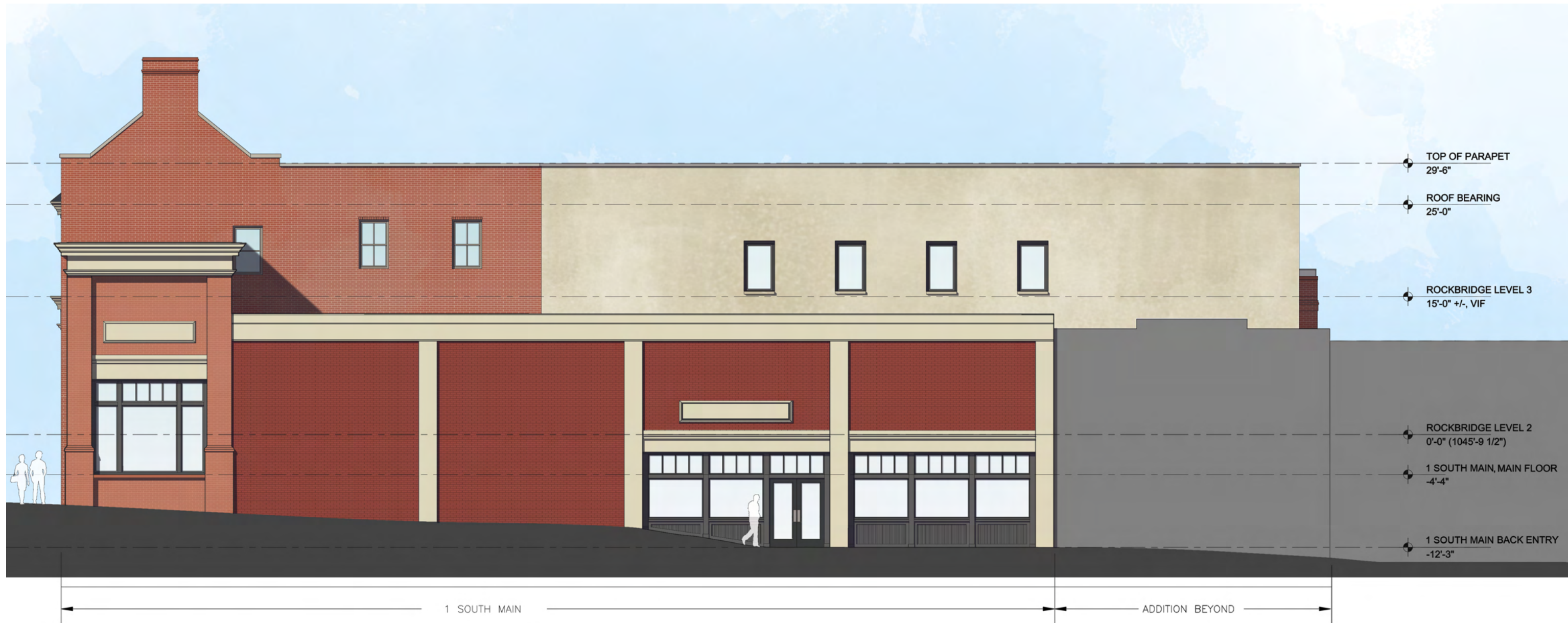
A1 EXTERIOR ELEVATION - NORTHEAST SCALE: 3/32" = 1'-0"
