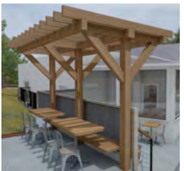
PERGOLA: 8'x12' with white oak 6x6 structural members and 2x6 shading members, natural finish.
