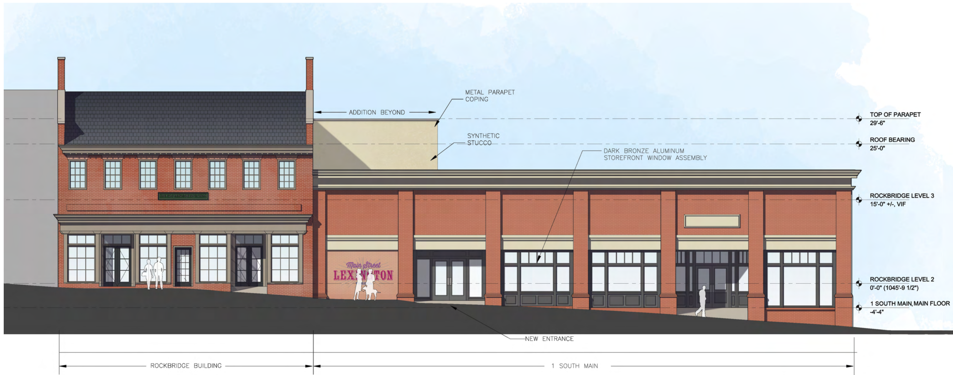
A1 EXTERIOR ELEVATION - SOUTHEAST SCALE: 3/32" = 1'-0"
